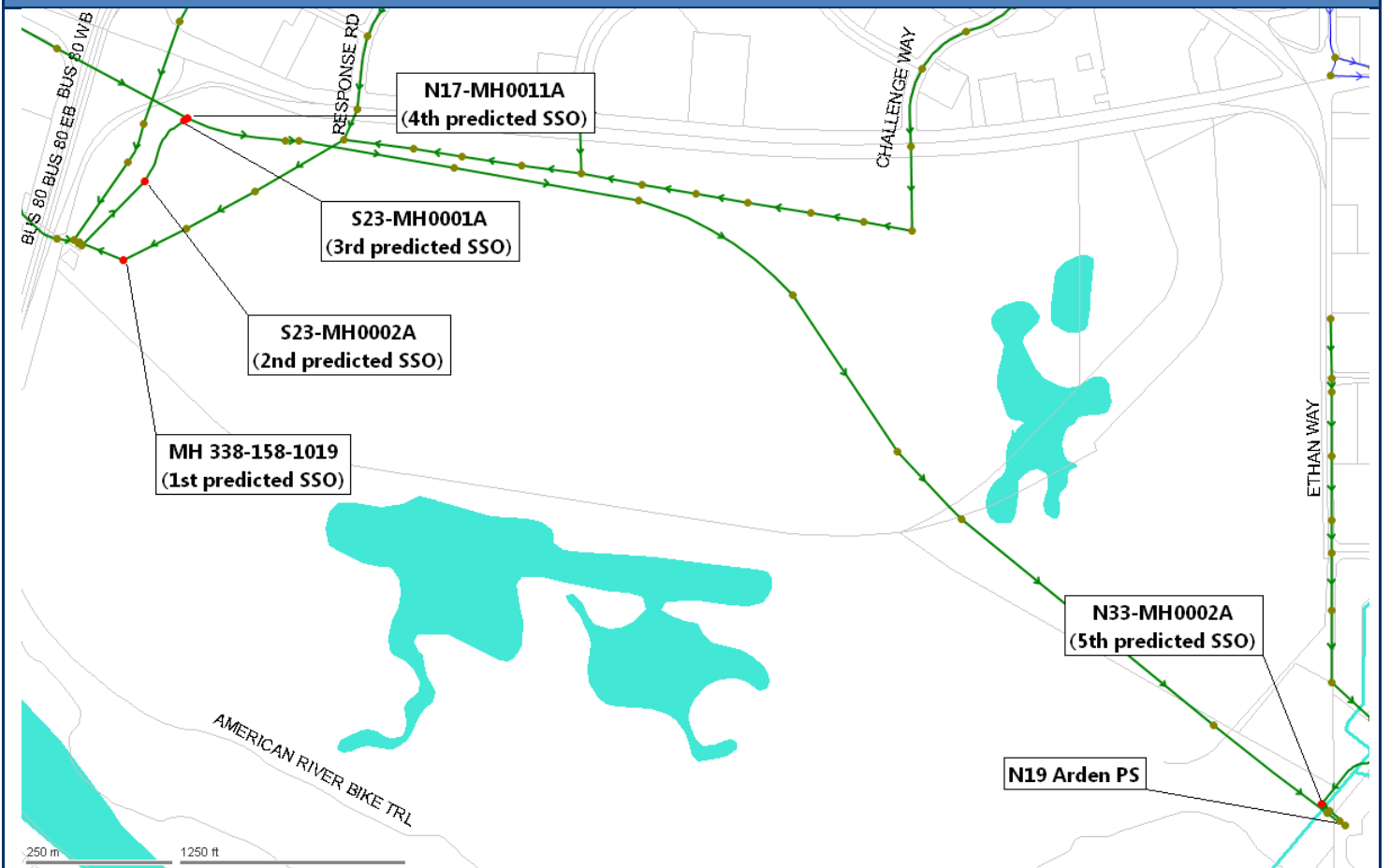
Figure 2: Map showing the location of the five model predicted overflows as a result of backed-up flow when the Arden Pump Station is not in operation.
